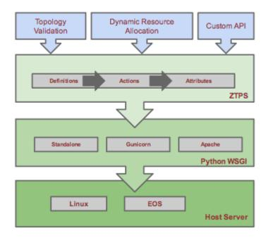
The server can run on any standard x86 server. Currently the only OS-es tested are Linux and MacOS, but theoretically any system that supports Python could run ZTPServer. The server provides a Python WSGI compliant interface, along with a standalone HTTP server. The built-in HTTP server runs by default on port 8080 and provides bidirectional file transport and communication for the bootstrap process.
