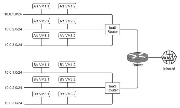
Besides, typical typologies can be combined to new typologies; for example, a flat network and a private network can be put together, as:
