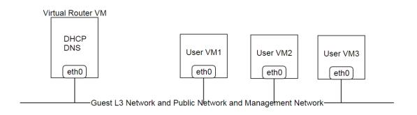
For a *private network or isolated network*, a virtual router VM provides DHCP, DNS, SNAT; and may provide EIP and Port Forwarding too, depending on users' choices; the network typologies can be:
