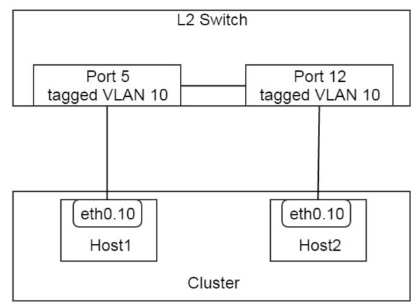
In this setup, two switch ports 5 and 12 are tagged with VLAN 10(trunk port with VLAN 10 in Cisco term), and respectively connect to eth0.10 that is a pre-created VLAN device on host1 and host2. This is also a very valid setup matching to a L2NoVlanNetwork. Admins can create a L2NoVlanNetwork with 'physicalInterface' = 'eth0.10' and attach it to the cluster.
