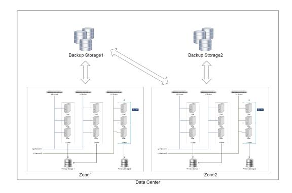
Note: For simplicity, the diagram omits some facilities like aggregation switches, core switches, routers, load bal-
