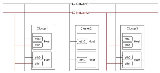
Let's assume the network typology in your datacenter is as above diagram. Eth0 of hosts in all clusters are on the same layer 2 network called L2 Network1; eth1 of cluster1 and cluster3 are on another layer 2 network called L2 network2. To describe this typology in ZStack, you can attach L2 network1 to all three clusters but attach L2 network2 to only cluster1 and cluster3.
