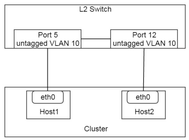
In this setup, two switch ports 5 and 12 are untagged with VLAN 10(access port with VLAN 10 in Cisco term), and connect to eth0 on host1 and host2 respectively. This is a very valid setup matching to a L2NoVlanNetwork. Admin cans create a L2NoVlanNetwork with 'physicalInterface' = 'eth0' and attach it to the cluster.
