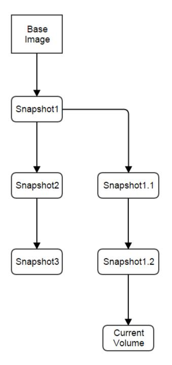
Current volume is always following the last snapshot; when a snapshot chain has too many delta snapshots, it may hurt the volume's disk IO performance, so ZStack sets max length of a snapshot chain to 16 by default; a new snapshot chain will be created after taking 16 snapshots.
