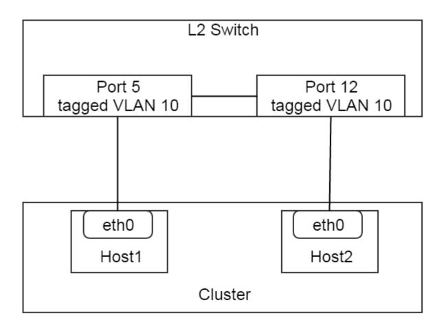
In this setup, switch ports 5 and 12 have been tagged with VLAN 10, then admins can create a L2VlanNetwork with 'physicalInterface' = 'eth0' and 'vlan' = 10 and attach it to the cluster.
