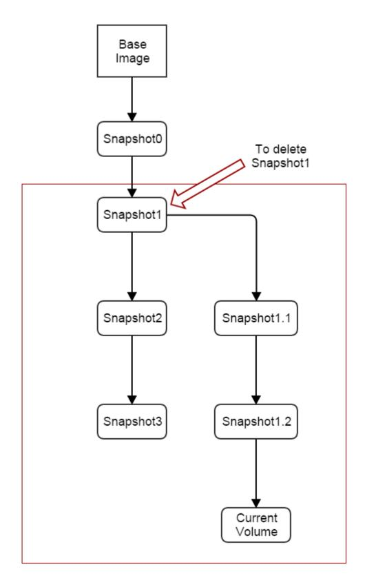
after deleting Snapshot1, the Snapshot2, Snapshot3, Snapshot1.1, and Snapshot1.2 will deleted too, and the snapshot chain turns to be:
