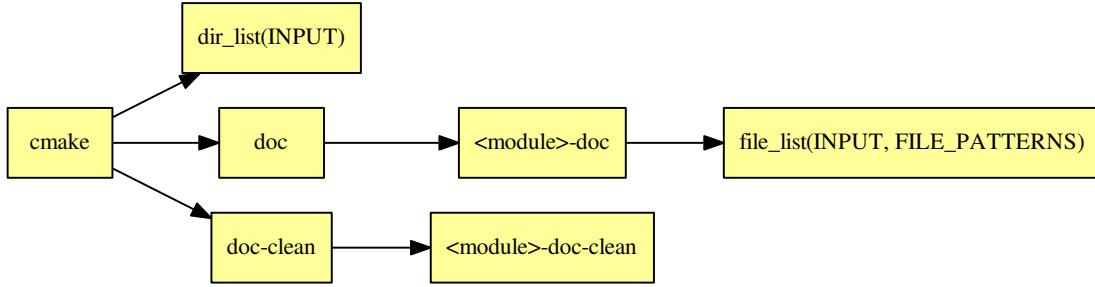
**Warning:** The dependency of cmake build system to the modification time of INPUT directories doesn't work with cmake versions prior to 3.0. This mean you must re-run cmake after adding new sources files in order to properly update the target files dependencies
