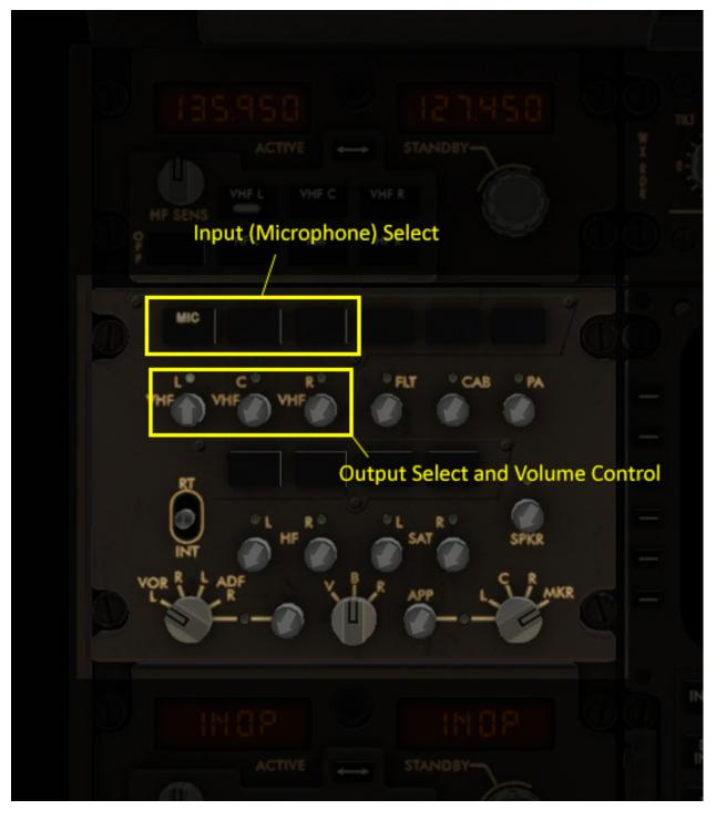
Fig. 2: X-Plane 11 audio controls in the Boeing 747-400 (Center Pedestal)
