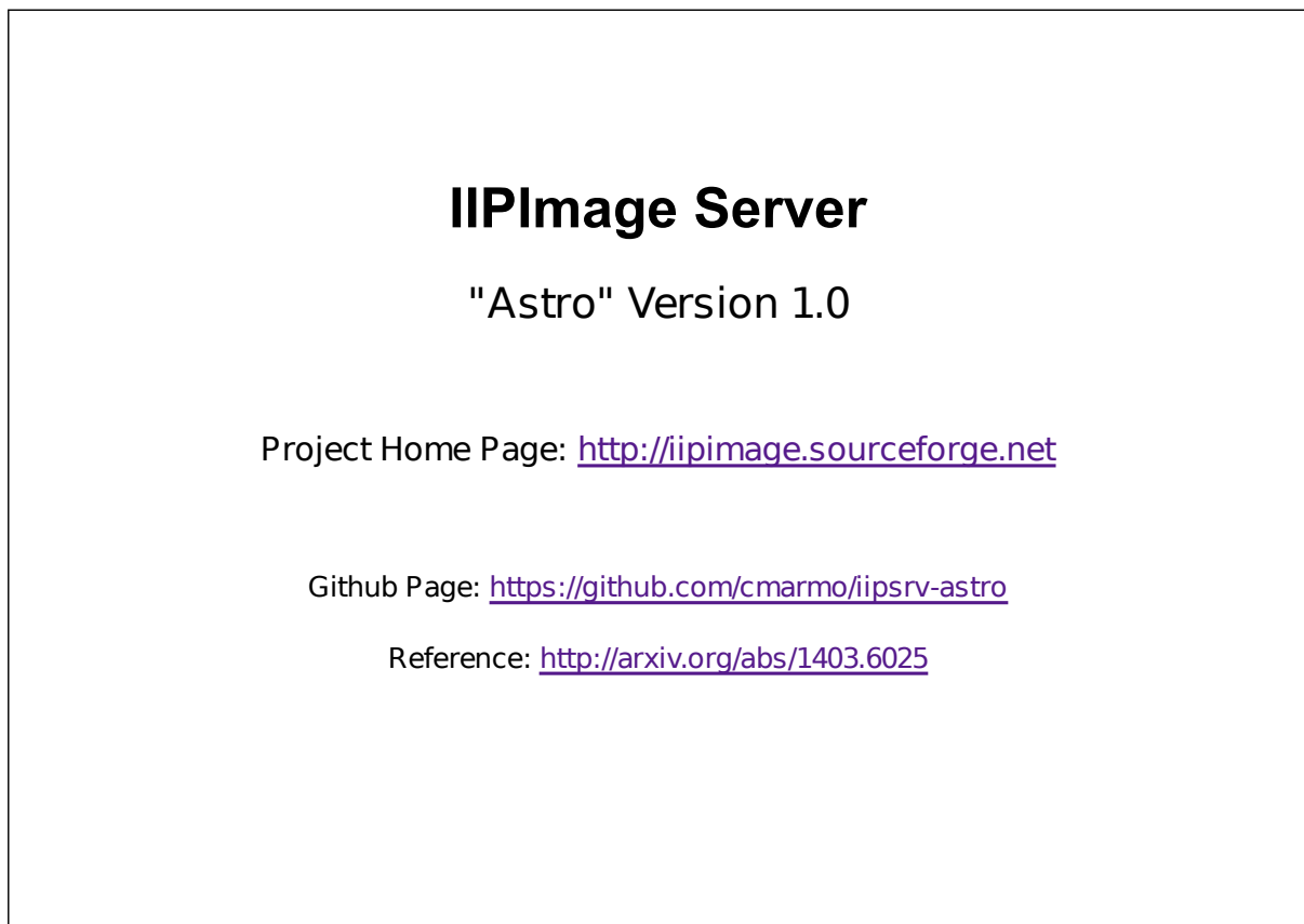
Fig. 6.6: Web page returned by the iipsrv CGI in the absence of arguments.
