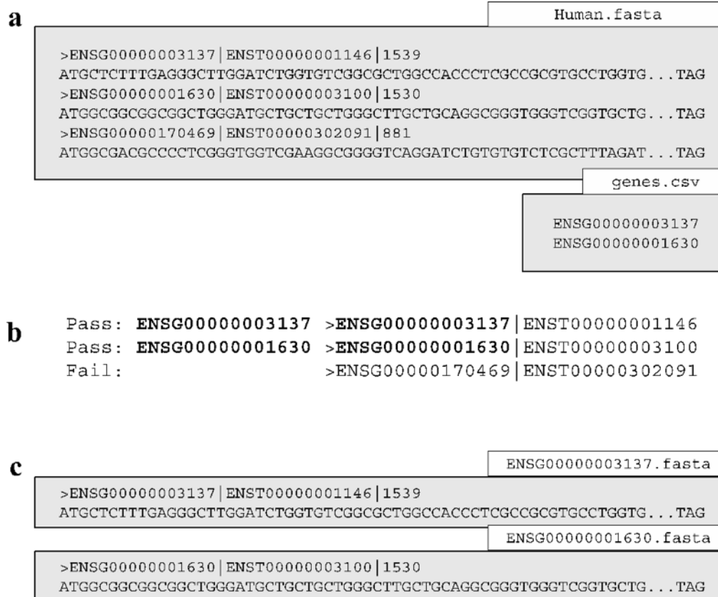
Fig. 1.4: FastA formatted files are shown as grey boxes and their filenames in white boxes. Data confirmation steps indicate if the results passed the check. (a) The gene_selection function requires two files to operate: a database (Human.fasta) and a user specified gene identifiers file (genes.csv). (b) The function operates using header confirmation to identify sequences in the database that match to those specified by the user. (c) The output of the function is a single sequence file for each user specified genes found.
