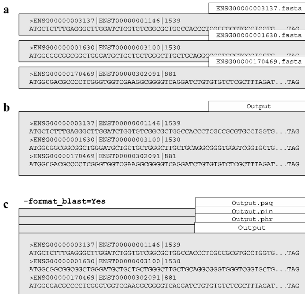
Fig. 1.3: Fasta formatted files are shown as grey boxes and their filenames in white boxes. Invoking the create_database function (a) combines numerous sequence files into (b) a single sequence database file. (c) Shows the format_blast option that will generate the required database files for BLAST [Altschul et al., 1990].
