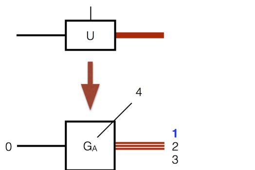
To obtain **G<sub>A</sub>**, **G<sub>B</sub>**, we need to multiply the bonds with  $\text{Ls}[i]^{-1}$
