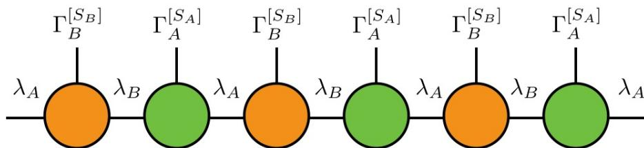
where  $\Gamma^{[A]_{S_A}}$  and  $\Gamma^{[B]_{S_B}}$  are  $\chi \times \chi$  matrices on the A and B sublattices, and  $\lambda^A$  and  $\lambda^B$  are Schmidt values.
