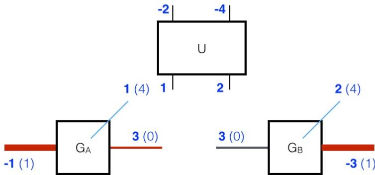
Performing SVD on  $\Theta$  and truncate the bond, we have three new tensors
