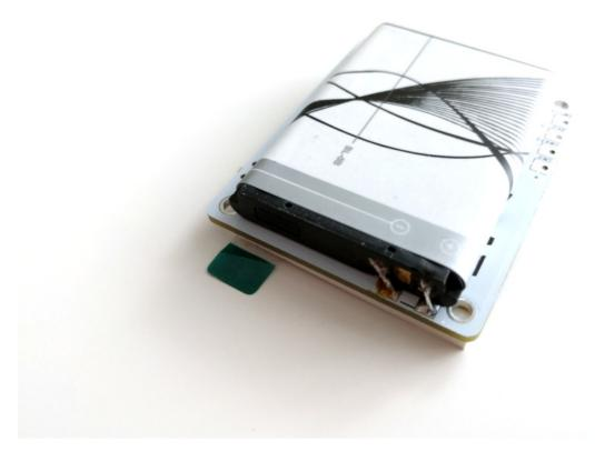
Note that different batteries have their terminals arranged differently, and that there is usually a third terminal with just a resistor connected to it, for battery identification — you don't need to connect that third terminal to anything. It's best to use a multimeter to make sure you got the connections right.
