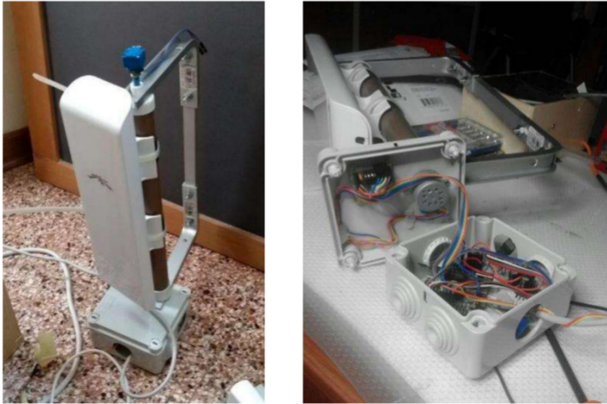
Fig. 2: Figure 3-2 The first version of the prototype of the Turnantenna
