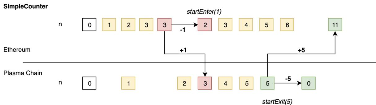
A yellow box means that the `counter()` has increased the status variable `n` by 1, a red box means entering the request changes `n`, and a green box means exiting the request changes `n`.
