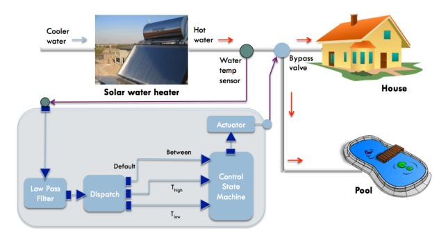
We see that the water sensor's output is run through a low pass filter to reduce noise in the reading. It is then passed to a dispatcher  $1[#]_$  which sends each event to one of several output ports, depending on how it compares to T\_low and T\_high. The control state machine determines when to turn on the actuator, based on the current state and the port of the input event.
