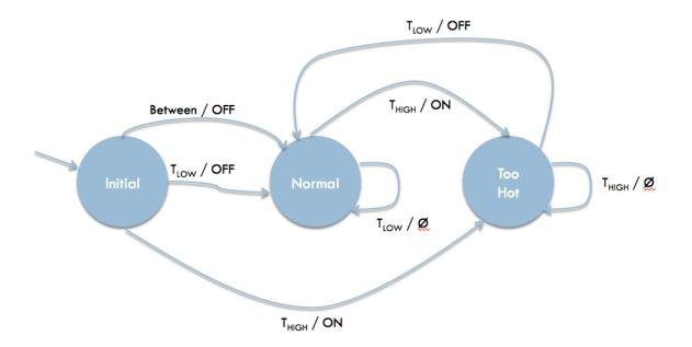
We start in the state Initial. If the first incoming event is T\_high, we go to the Normal state. Othewise, we immediately go to Too Hot, which will turn off the actuator. After the initial event, we move from Normal to Too Hot if we receive a T\_high event and then back to Normal when we receive T\_low. Here is the code which implements this state machine as a ThingFlow filter:
