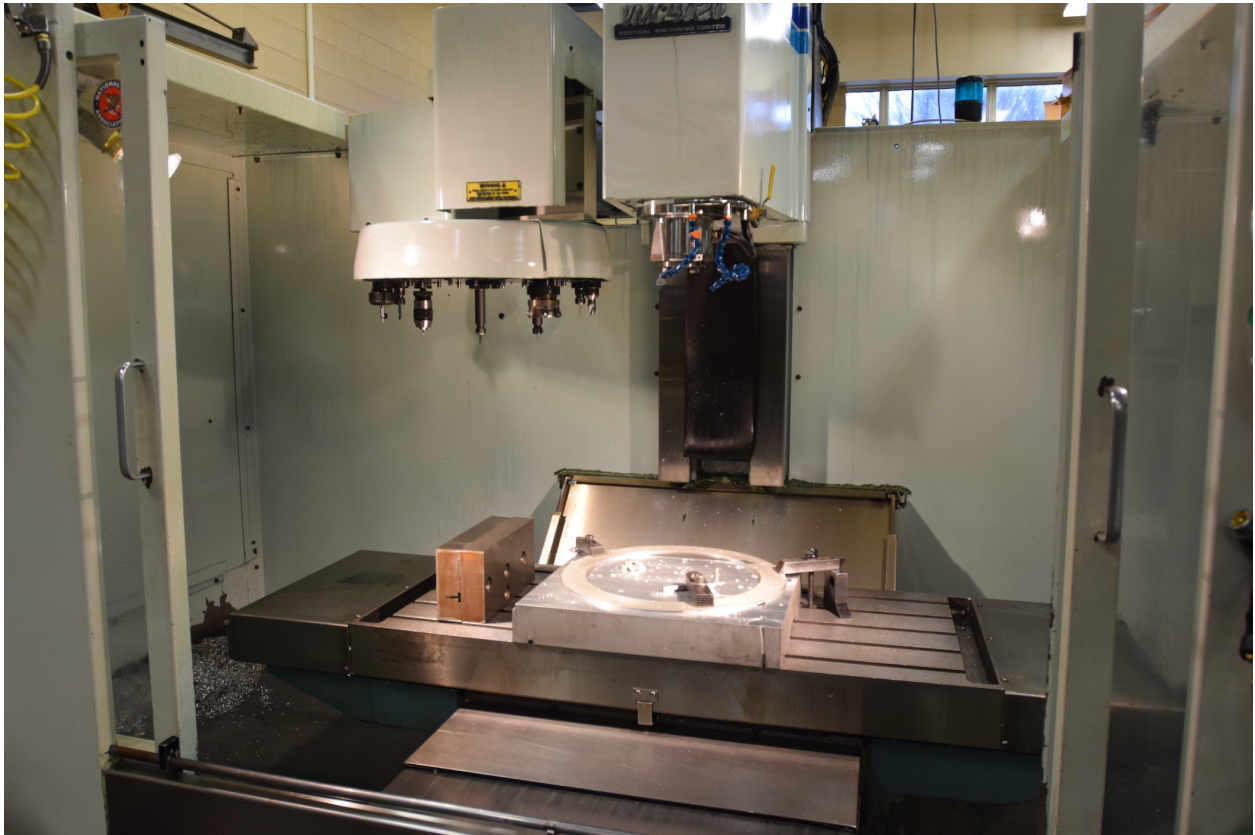
Fig. 1.39: A CNC milling machine with tool changer (Ellis Dunklebarger)
