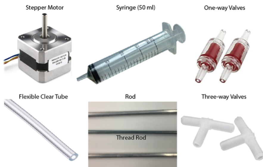
Figure 3. Major hardware component of syringe pump system
