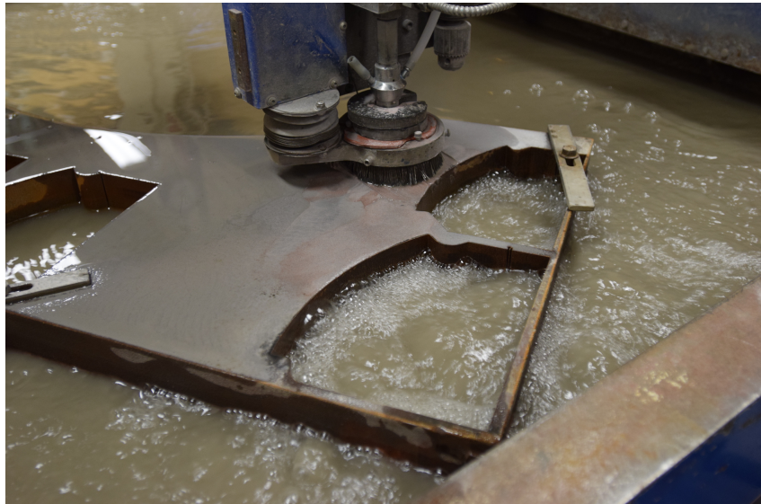
Fig. 1.40: Waterjet cutting a thick steel plate (Ellis Dunkleberger)
