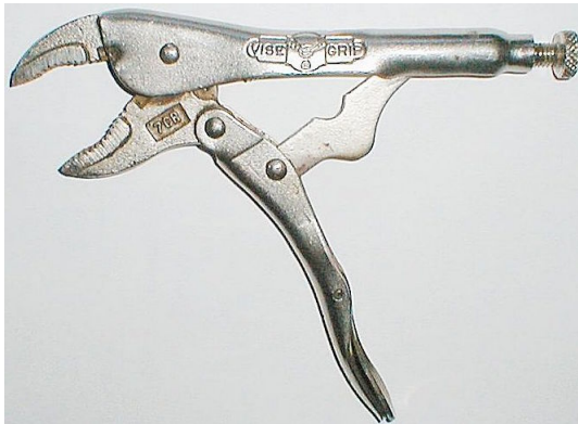
Fig. 1.10: Locking Pliers (Wikipedia)
