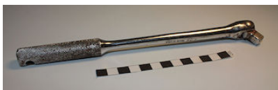
Fig. 1.27: Breaker Bar (Wikipedia)
