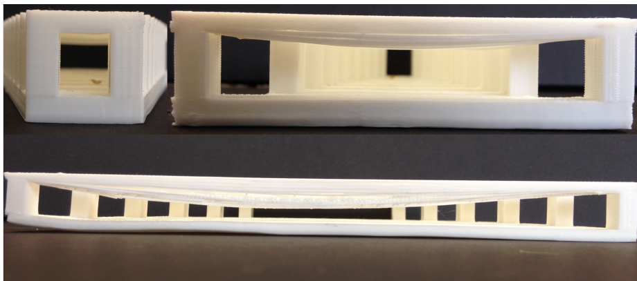
Clockwise from top left \leq 36\text{mm} – 0-0.5mm drooping, 36-60mm – 0.5-2mm drooping, \geq 60\text{mm} – 2-5mm drooping
