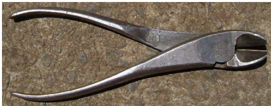
Fig. 1.7: Diagonal Cutters (Wikipedia)
