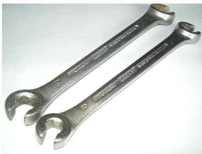
Fig. 1.24: Flare Nut Wrench (Wikipedia)
