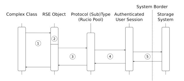
**1. Interaction Request:** Whenever a complex class wants to interaction with the specified storage, it uses one of the operations provided by the RSE object. This operation could be for example GET a file, GET a directory listing, DELETE a file, ... A detailed discussion about the provided operations is given in the according section later in this document.
