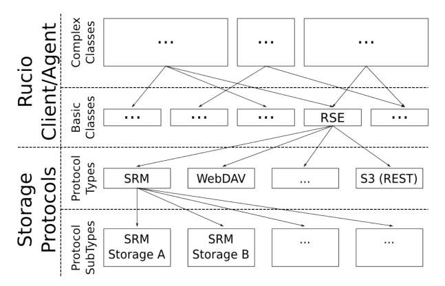
Because some storages use the same protocol, a Rucio-wide pool of protocol implementations for the system is also provided. What protocols (cloud be more than one) are supported by a specific storage is defined in its according properties (RSEProperties). Unfortunately, different version/implementations of one protocol, which differ in various ways, are implemented by the different storages. Due to re-usability reasons we therefore decided to allow various
