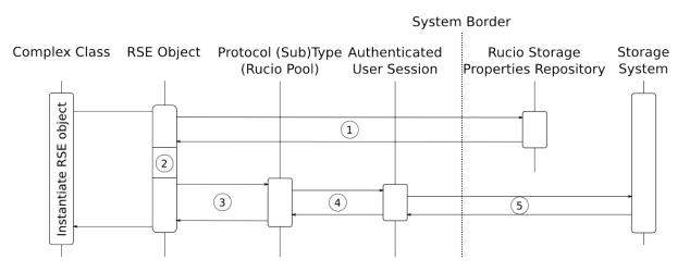
Whenever an interaction with a storage is requested, an RSE object has to be instantiated. The illustration above gives an overview about what happens at run-time during its instantiation.
