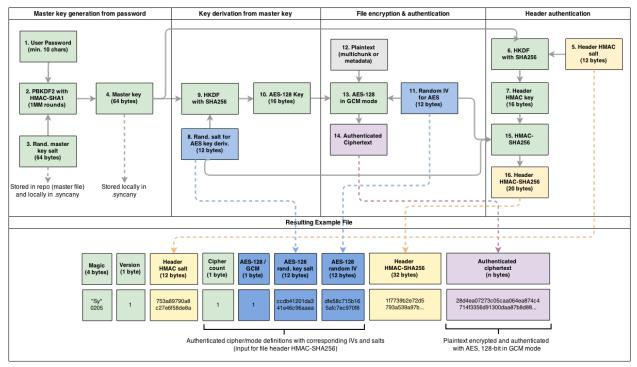
The diagram shows an example for the default configuration: For each file to be encrypted, Syncany uses **HKDF with SHA-256** and a **random 96-bit salt** to derive a **128-bit file key** to use for the AES cipher (8-10). In addition to that, a **128-bit random IV** is created and used as input for the cipher (11). Using the 128-bit key and the 128-bit IV, Syncany then encrypts plaintext (= multichunk file, database file, etc.) using the AES cipher in GCM mode.
