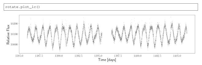
Now let's measure a rotation period for this star using the astropy implementation of the Lomb-Scargle periodogram. This algorithm fits a single sinusoid to the light curve and reports the squared amplitude of the sinusoid over a range of frequencies (1/periods).
