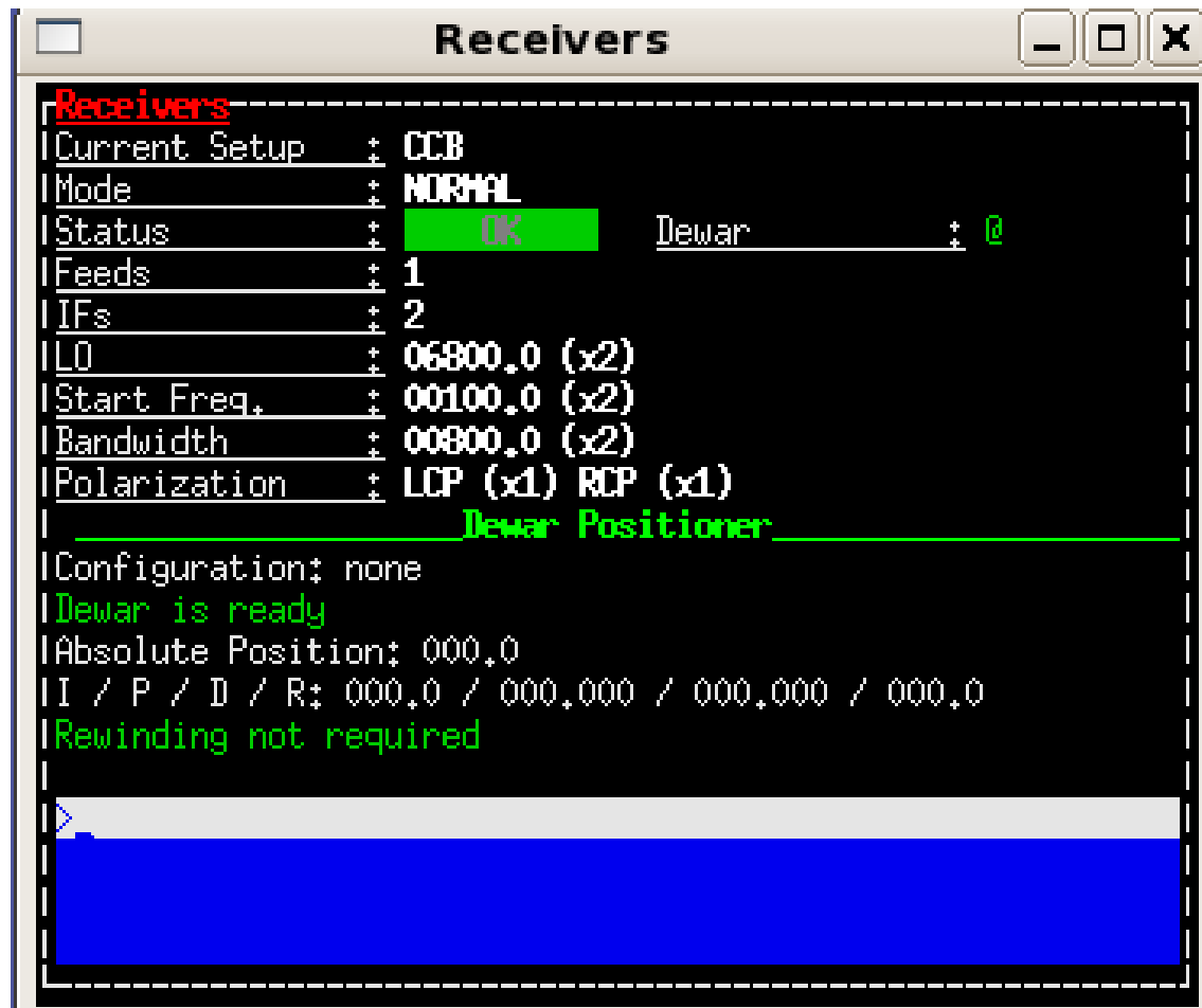
Fig.4.18: The ReceiverBoss monitor summarizes the frontend setup parameters. The bottom part is devoted to the derotator (dewar positioner), when available.
