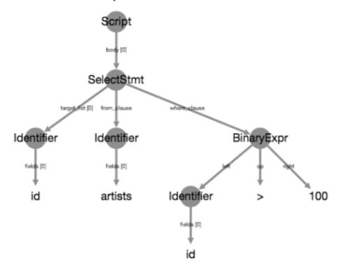
• Next, check\_node() chains off of the state produced by Ex() and produces a child state that focuses on the SelectStmt portion of the submission and solution:
