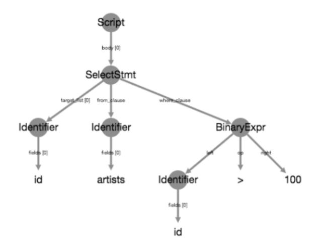
Notice how the statement is neatly chopped up into its consituents: the SELECT statement is chopped up into three parts: the target\_list (which columns to select), the from\_clause (from which table to select) and the where\_clause (the condition that has to be satisfied). Next, the where\_caluse is a BinaryExpr that is further chopped up.
