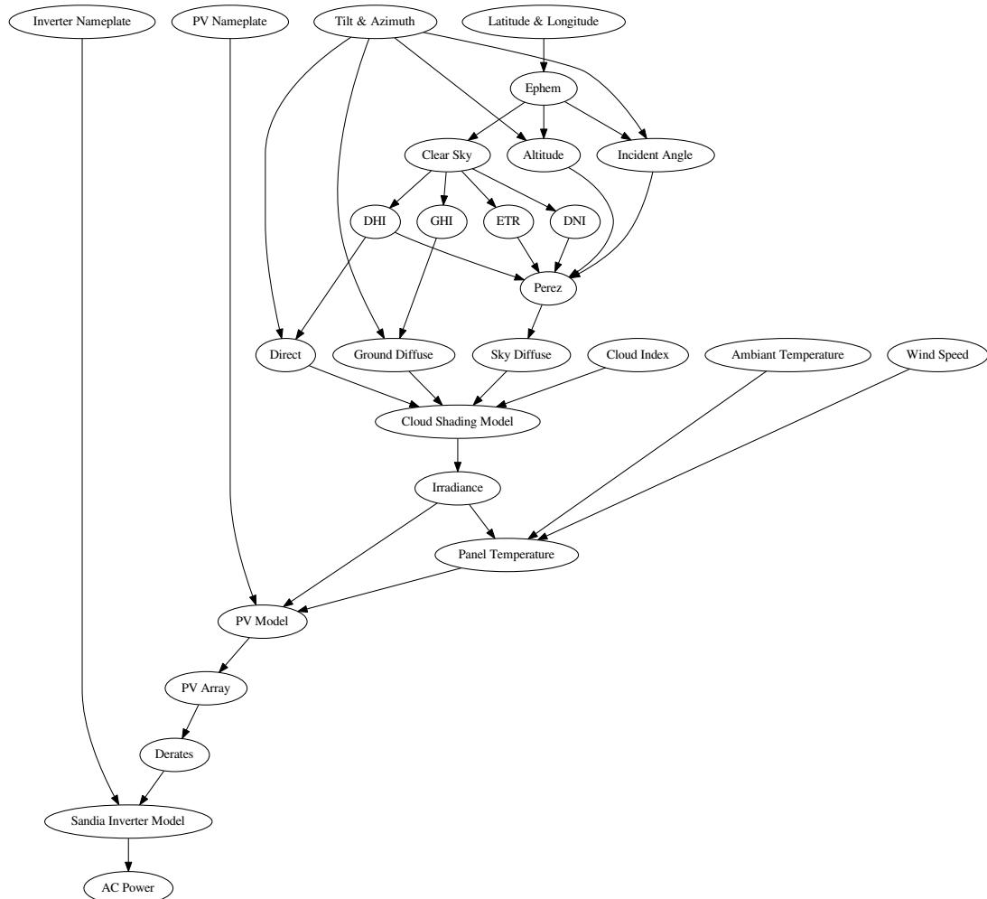
This graph shows the interaction of models. Models can be connected to interact in different ways. For example shading obstructions can be applied after irradiance has been calculated. This is the method some tools in the solar industry such as the Solar Pathfinder use to simplify the process. However it can be applied earlier to better estimate diffuse and reflected components.
