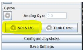
To configure a I2C or SPI device, click on the SPI & I2C button
