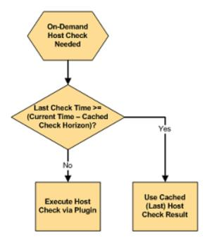
When Shinken needs to perform an on-demand host or service check, it will make a determination as to whether it can used a cached check result or if it needs to perform an actual check by executing a plugin. It does this by checking to see if the last check of the host or service occurred within the last X seconds, where X is the cached host or service check horizon.
