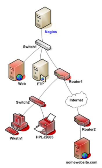
In this example, Shinken will determine that Web and Router1 are both in DOWN states because the "path" to those hosts is not being blocked (switch1 is still alive), and so it will allow web and router1 notifications to be sent.
