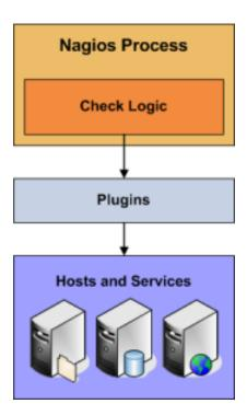
Active checks are initiated by the check logic in the Shinken daemon. When Shinken needs to check the status of a host or service it will execute a plugin and pass it information about what needs to be checked. The plugin will then check the operational state of the host or service and report the results back to the Shinken daemon. Shinken will process the results of the host or service check and take appropriate action as necessary (e.g. send notifications, run event handlers, etc).
