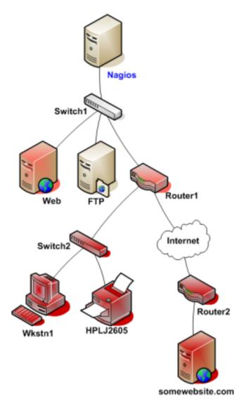
In this example, Shinken will determine that Web and Router1 are both in DOWN states because the "path" to those hosts is not being blocked.
