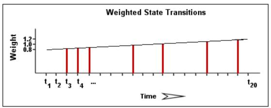
Using the images above, lets do a calculation of percent state change for the service. You will notice that there are a total of 7 state changes (at t3, t4, t5, t9, t12, t16, and t19). Without any weighting of the state changes over time, this would give us a total state change of 35%:
