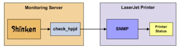
Monitoring the status of a networked printer is pretty simple. JetDirect-enabled printers usually have "SNMP" enabled, which allows Shinken to monitor their status using the **check\_hpjd** plugin.
