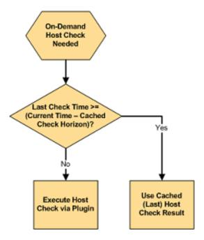
When Shinken needs to perform an on-demand host or service check, it will make a determination as to whether it can used a cached check result or if it needs to perform an actual check by executing a plugin. It does this by checking to see if the last check of the host or service occured within the last X seconds, where X is the cached host or service check horizon.
