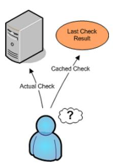
The performance of Shinken' monitoring logic can be significantly improved by implementing the use of cached checks. Cached checks allow Shinken to forgot executing a host or service check command if it determines a relatively recent check result will do instead.
