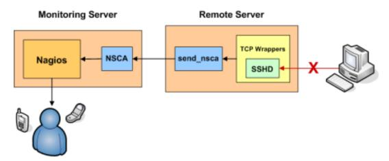
This document explains how to easily generate alerts in Shinken for connection attempts that are rejected by TCP wrappers. For example, if an unauthorized host attempts to connect to your "SSH" server, you can receive an alert in Shinken that contains the name of the host that was rejected. If you implement this on your Linux/Unix boxes, you'll be surprised how many port scans you can detect across your network.
