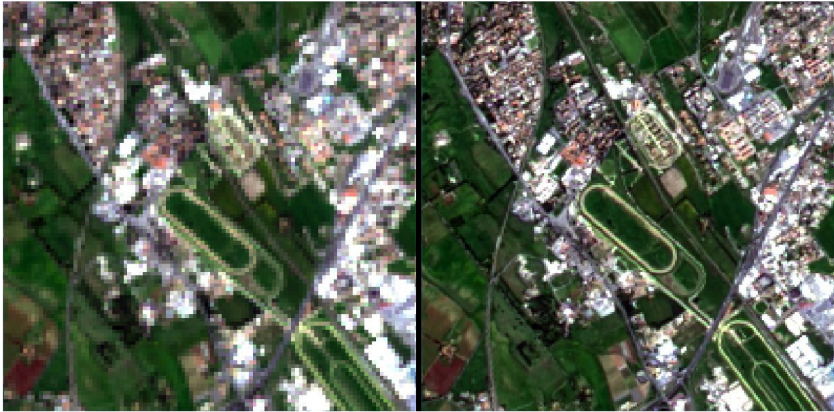
Rys. 14.4: Example of pan-sharpening of a Landsat 8 image. Left, original multispectral bands (30m); right, pan-sharpened bands (15m)
