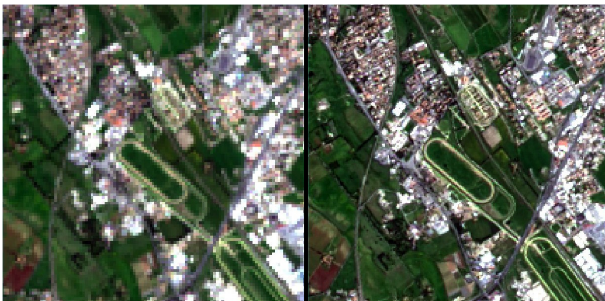
Figure 13.4: Example of pan-sharpening of a Landsat 8 image. Left, original multispectral bands (30m); right, pan-sharpened bands (15m)
