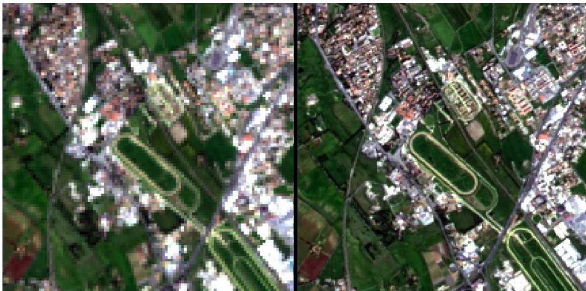
Rys. 12: Example of pan-sharpening of a Landsat 8 image. Left, original multispectral bands (30m); right, pan-sharpened bands (15m)
