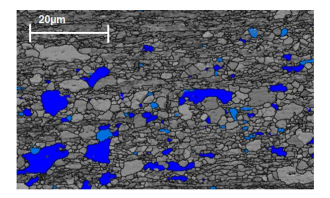
Band contrast SEM/EBSD image of an electropolished AA8079 sample after 70% cold-rolling and isothermal annealing at 300 deg C for 6 minutes. .. The rolling direction is parallel to the scale bar. Blue denotes grains in cube orientation, high-angle grain boundaries drawn in black.
