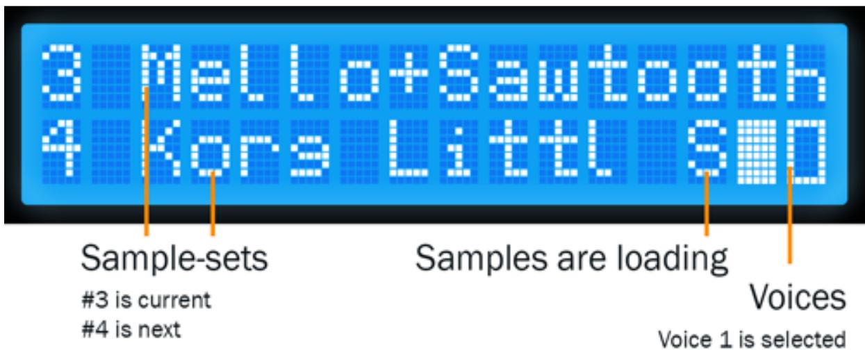
Displaying current preset '3 Mello+Sawtooth' which has 2 voices available. The next preset is '4 Korg Little Bits'. The 'S' indicates samples are still loading in the background
