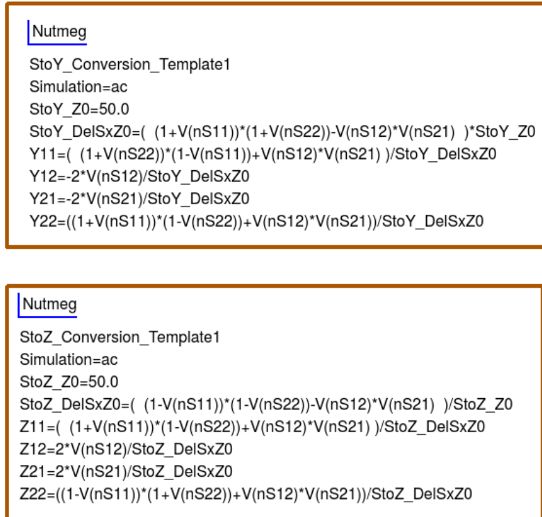
Figure 13.5 Qucs-S Nutmeg equation block templates for S to Y and Z parameter conversion.
