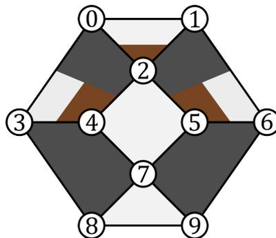
In this figure we see an example stabilizer code. Data qubits are indicated as white circles and are labelled by numbers. Polygons represent checks. The coloring of the polygons indicate how the associated check acts on qubits it touches. When the check is white on a qubit, the check acts as  $Z$ . When black,  $X$ . When brown,  $Y$ .
