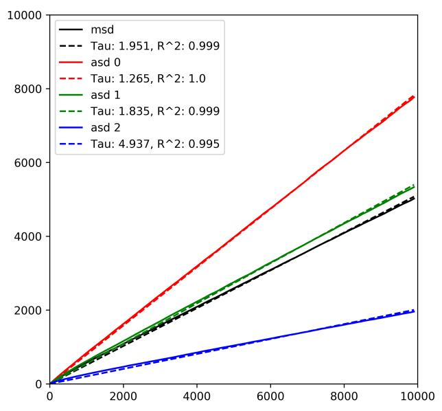
Unlike the previous examples, the MSD plot clearly shows that the axial square displacement is different along the different axes and this produces a tortuosity that approximately scales with the blobiness of the image. The image is three-dimensional and so we cannot use the 2D plotting function to visualize the walks, instead we make use of the export function to produce a set of files that can be read with Paraview:
