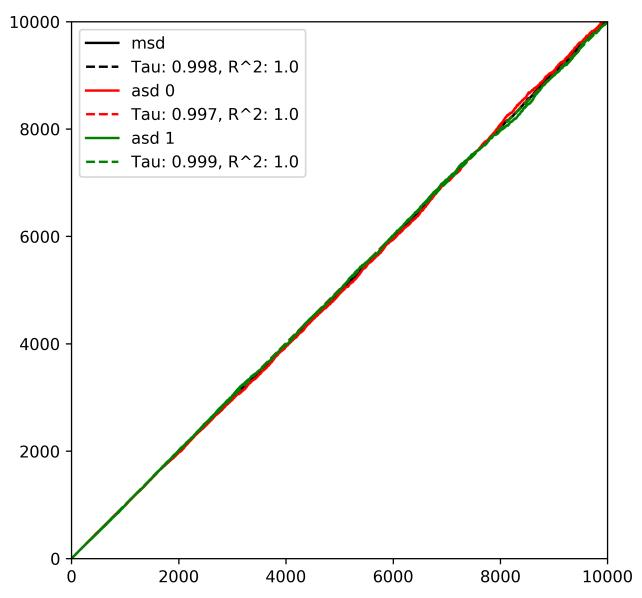
The plot\_msd function shows that mean square displacement and axial displacement are all the same and increase linearly with time. A neat explanation of why this is can be found in this paper http://rsif.royalsocietypublishing.org/ cgi/doi/10.1098/rsif.2008.0014 which derives the probability debnsity function for the location of a walker after time t as:
