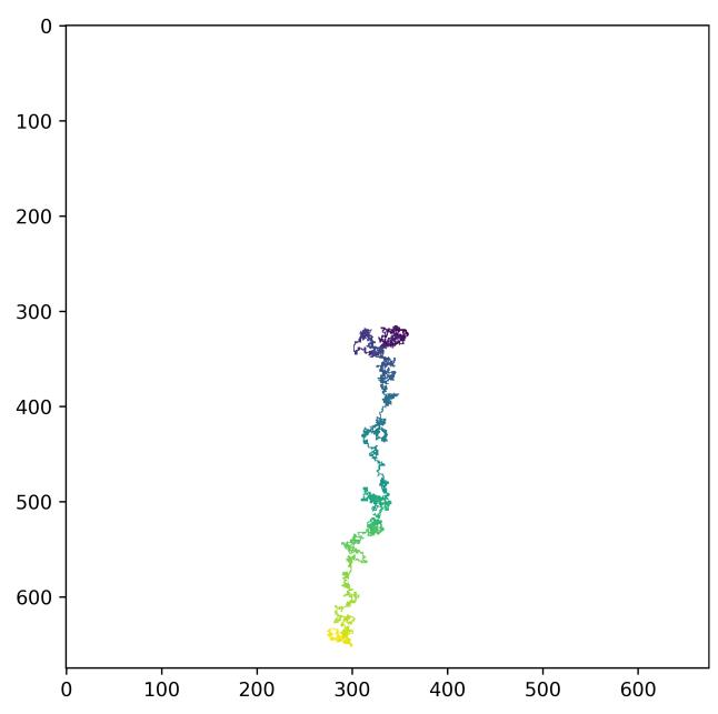
The attribute  $rw.sq_disp$  is the square displacement for all walkers at all stride steps which is all steps for this example. Indexing -1 takes the last row and indexing : takes the whole row, the numpy function argmax returns the index of the largest value and this integer value is used for the w\_id argument of the plotting function which stands for walker index.
