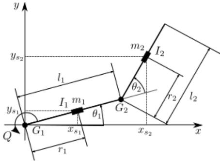
The modeling was taken from the thesis of Carsten Knoll (April, 2009) where in addition the inertia parameter  $\eta$  was introduced.
