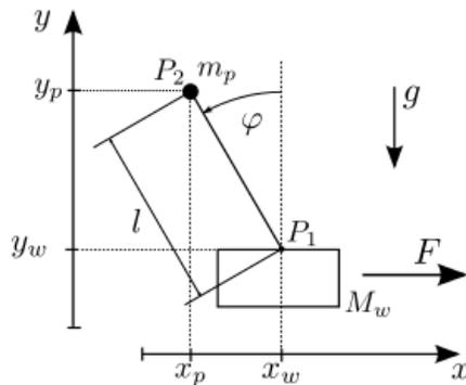
With the *Lagrangian Formalism* the model has the following state representation where  $u_1 = F$  and  $x = [x_1, x_2, x_3, x_4] = [x_w, \dot{x}_w, \varphi, \dot{\varphi}]$
