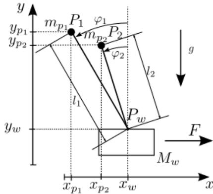
The system has the state vector  $x = [x_1, \dot{x}_1, \varphi_1, \dot{\varphi}_1, \varphi_2, \dot{\varphi}_2]$ . A partial linearization with  $y = x_1$  yields the following system state representation where  $\tilde{u} = \ddot{y}$ .
