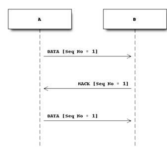
For each DATA frame sent, a timer is started. If the timer ends before receiving any corresponding ACK and NACK frame, the DATA frame will be sent again:
