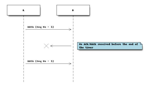
The default timer value is 2 seconds and can be changed using the sending\_timeout parameter of *HDLController*.
