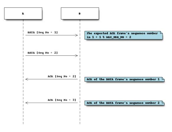
The number of DATA frames that can be sent before receiving the first acknowledgment is determined by the window parameter of *HDLController*. Its default value is 3.
