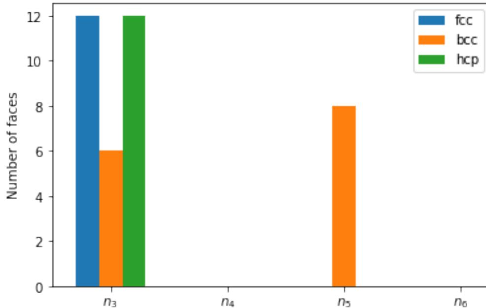
The difference in Voronoi fingerprint for bcc and the closed packed structures is clearly visible. Voronoi tessellation, however, is incapable of distinction between fcc and hcp structures.
