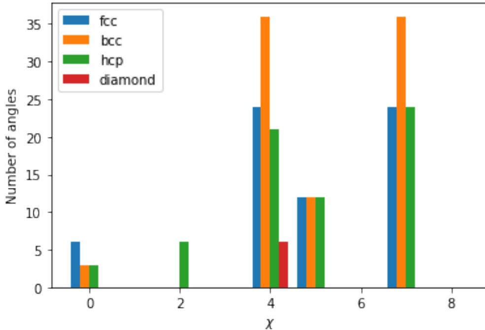
The atoms exhibit a distinct fingerprint for each structure. Structural identification can be made up comparing the ratio of various  $\chi$  parameters as described in the [original publication](#).
