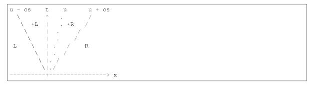
We care about the solution on the axis. The basic idea is to use estimates of the wave speeds to figure out which region we are in, and: use jump conditions to evaluate the state there.
