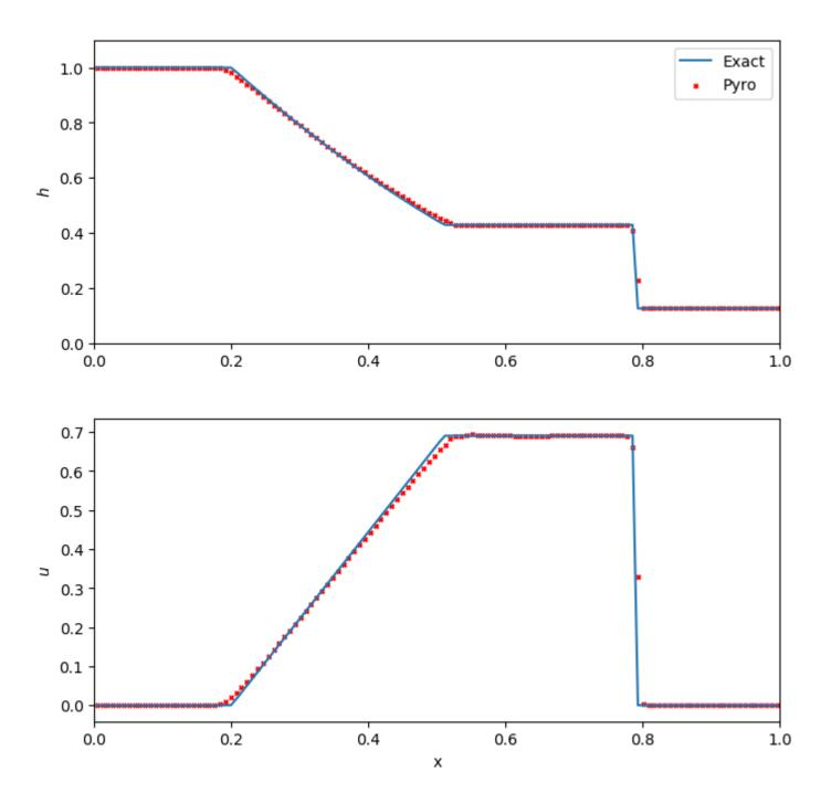
We see excellent agreement for all quantities. The shock wave is very steep, as expected. For this problem, the Roe-fix solver performs slightly better than the HLLC solver, with less smearing at the shock and head/tail of the rarefaction.
