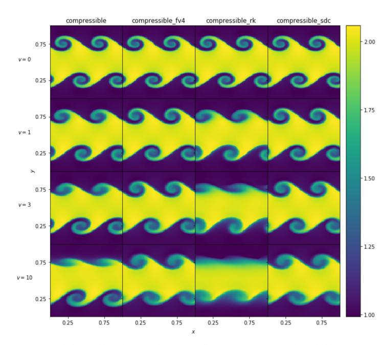
We vary the velocity in the positive y-direction (vbulk) to see how effective the solvers are at preserving the initial shape.
