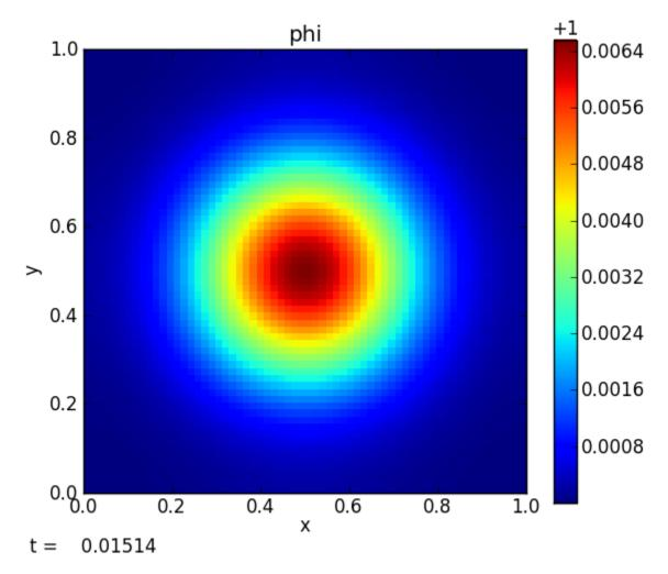
The above figure shows the scalar field after diffusing significantly from its initial strongly peaked state. We can compare to the analytic solution by making radial profiles of the scalar. The plot below shows the numerical solution (red points) overplotted on the analytic solution (solid curves) for several different times. The y-axis is restricted in range to bring out the detail at later times.
