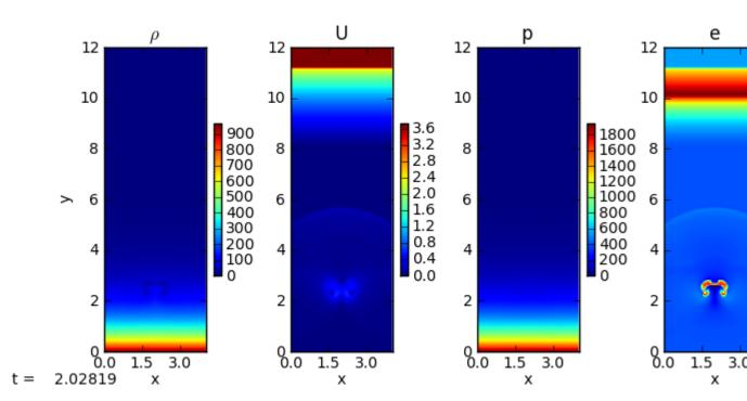
The shock at the top of the domain is because we cut off the stratified atmosphere at some low density and the resulting material above that rains down on our atmosphere. Also note the acoustic signal propagating outward from the bubble (visible in the U and e panels).
