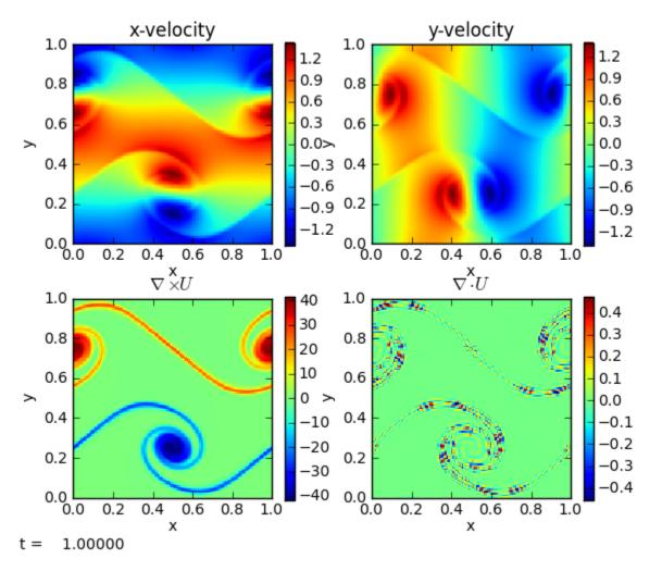
The vorticity panel (lower left) is what is usually shown in papers. Note that the velocity divergence is not zero—this is because we are using an approximate projection.
