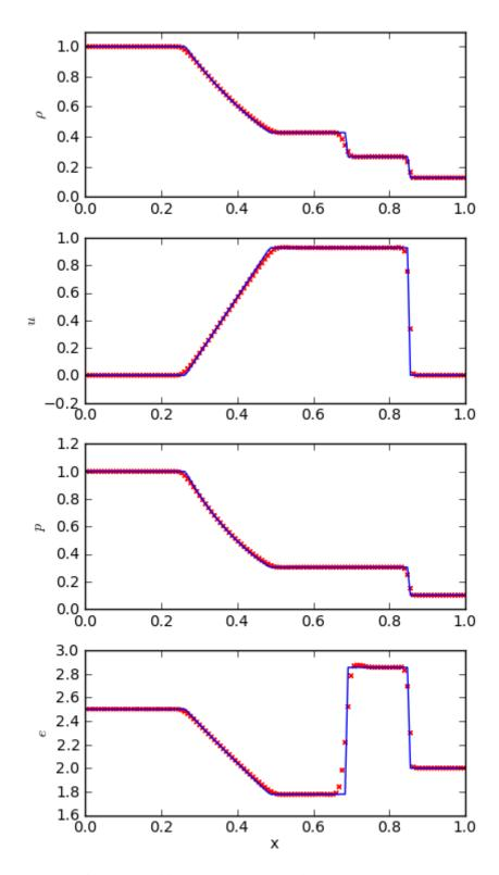
We see excellent agreement for all quantities. The shock wave is very steep, as expected. The contact wave is smeared out over ~5 zones—this is discussed in the notes above, and can be improved in the PPM method with contact steepening.
