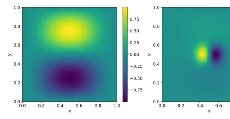
Left is the original u velocity, middle is the modified field after adding the gradient of the scalar, and right is the recovered field.
