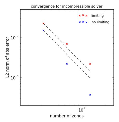
The dashed line is second order convergence. We see almost second order behavior with the limiters enabled and slightly better than second order with no limiting.
