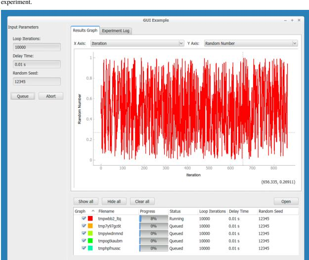
on the queue. In this context, the Manager uses an Experiment object to keep track of the Procedure, Results, and its associated graphical representations in the browser and live-graph. This is then given to the Manager to queue the experiment.
