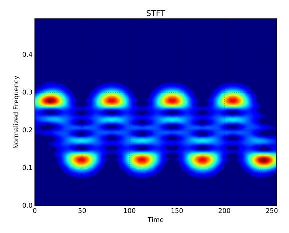
From this representation, the sinusoidal nature of the frequencies can be made out, and even the concentration of energy at the extrema of the sine wave makes sense. But the artifacts between the high energy areas are quite ambiguous, and bear little resemblance to the signal's true characterisitcs.
