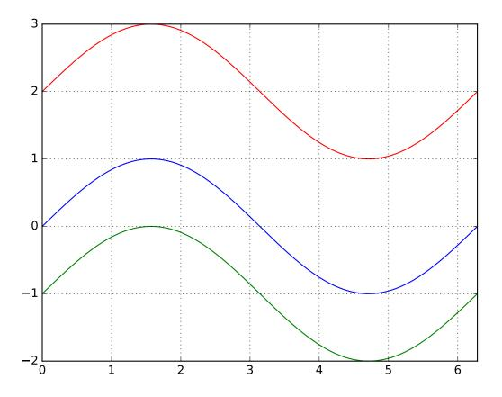
All of them are identical, except that two of them have a nonzero DC component. Since the Hilbert transform of sine is cosine, the analytic signals of these sinusoids should represent unit circles in the complex plane:
