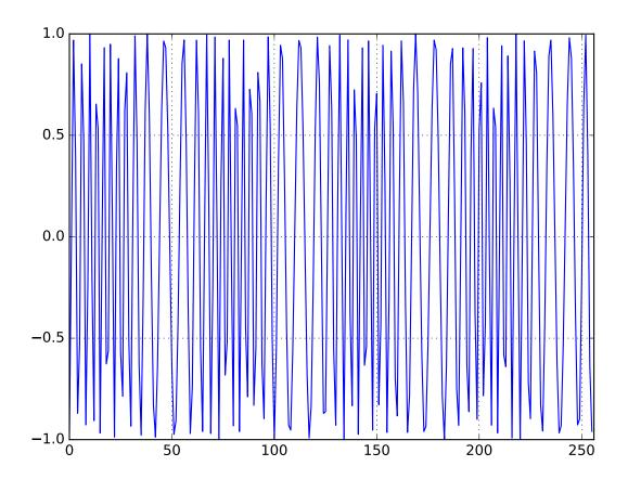
This signal contains frequencies which are modulated such that they vary sinusoidally between 0.1 and 0.3. The time-frequency distribution of this signal should look somewhat like a sine wave. Here's the spectrogram of the STFT of this signal:
