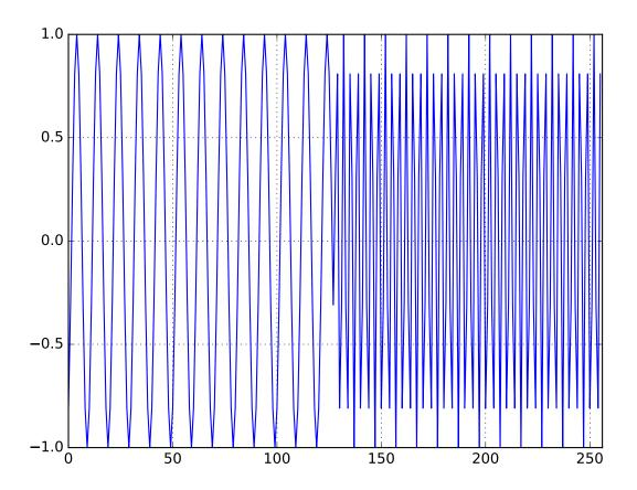
This first half of the signal is a sinusoid with a normalized frequency of 0.1 and the other half has a normalized frequency of 0.3. If we look at the energy spectrum of this signal, sure enough, there are two peaks at the respective frequencies:
