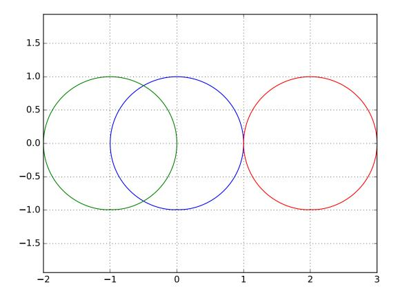
Imagine that each circle is traced out by a phasor rotating anticlockwise, which is centered at the origin in the figure above. The angle that the phasor rotates through in an infinitesimally small time period represents the instantaneous phase of the signal, and its time differential is the instantaneous frequency. Using this interpretation, let's try to compute the instantaneous frequencies of the three signals:
