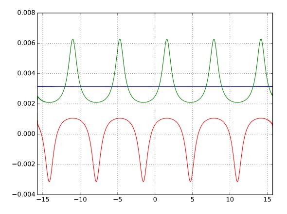
As shown in the figure, only one sinusoid presents an instantaneous frequency that is constant and corresponds to the true frequency of the waves. This wave is the one which has its analytical signal centered around the origin, thereby allowing the phasor to rotate through a total angle of  $2\pi$  in one period. This is the wave that has a zero DC component and is symmetrical around the time axis.
