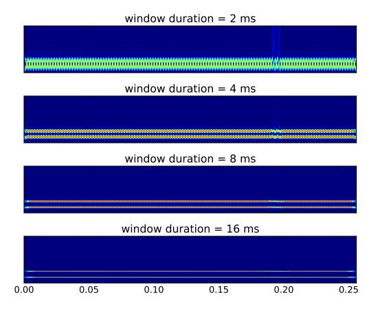
As can be clearly seen, resolution in time and frequency cannot be obtained simultaneously. In the last (bottom) image, where the window length is high, the STFT manages to discriminate between frequencies of 500 Hz and 1000 Hz very clearly, but the time resolution between the events at t = 0.192 s and t = 0.196 s is ambiguous. As we reduce the length of the window function, the resolution between the time events goes on becoming better, but only at the cost of resolution in frequencies.
