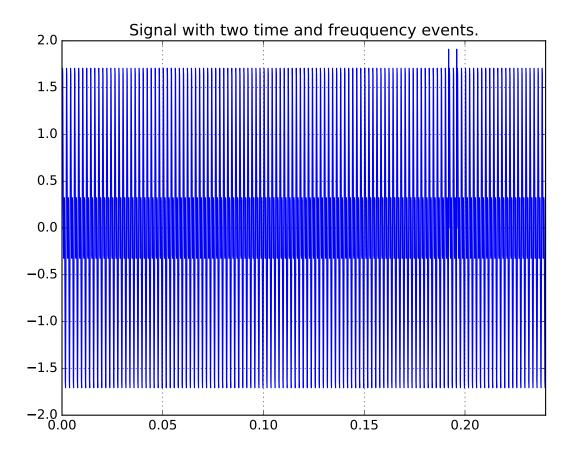
It is a sum of two sinusiodal signals of frequencies 500 Hz and 1000 Hz. It has two spikes at t = 0.192s and t = 0.196s. The purpose of a time frequency distribution would be to clearly identify both the frequencies and both the spikes, thus resolving events in both frequency and time. Let's check out the spectrograms of the STFTs of the signal with four different window lengths:
