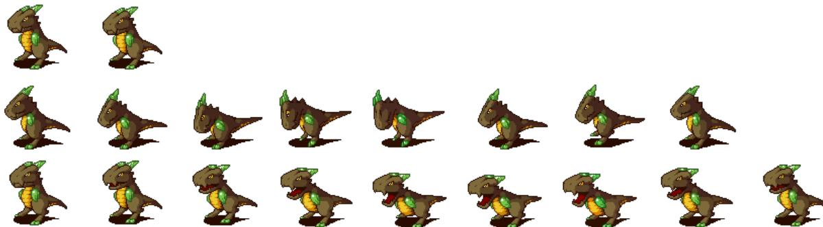
Sprites sheets can be loaded into a PygAnimation object without having to slice the sheet up into individual image files. The sprite sheet’s filename is passed to the `getImagesFromSpriteSheet()`, which returns a list of `pygame.Surface` objects.
