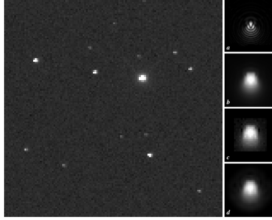
Fig. 1.6: Left : part of a simulated star field image with strong undersampling. Right, from top to bottom : (a) simulated optical PSF, (b) simulated PSF convolved by the pixel response, (c) PSF recovered by PSFEx at 4.5 times the image resolution from a random sample of 212 stars extracted in the simulated field above, using the “pixel” vector basis, and (d) PSF recovered using the “shapelet” basis with n_{\max} = 16 .
