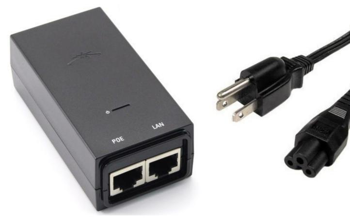
After plugging the adapter to a power outlet, the PoE port connects to the Bullet, while the LAN port connects to the Raspberry Pi's Ethernet port. In the Platypus boat, the connection is the same, except for the power which comes from the boat's electronics board, as shown in the diagram below:
