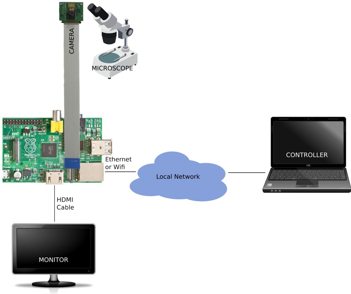
The Raspberry Pi's camera is attached to the microscope. The exact manner in which the camera is mounted is left as an exercise for the reader. Simply taping the camera onto the eye-piece with electrical tape is usually sufficient for testing, but better results are generally obtained when the camera is held slightly away from the eye-piece.
