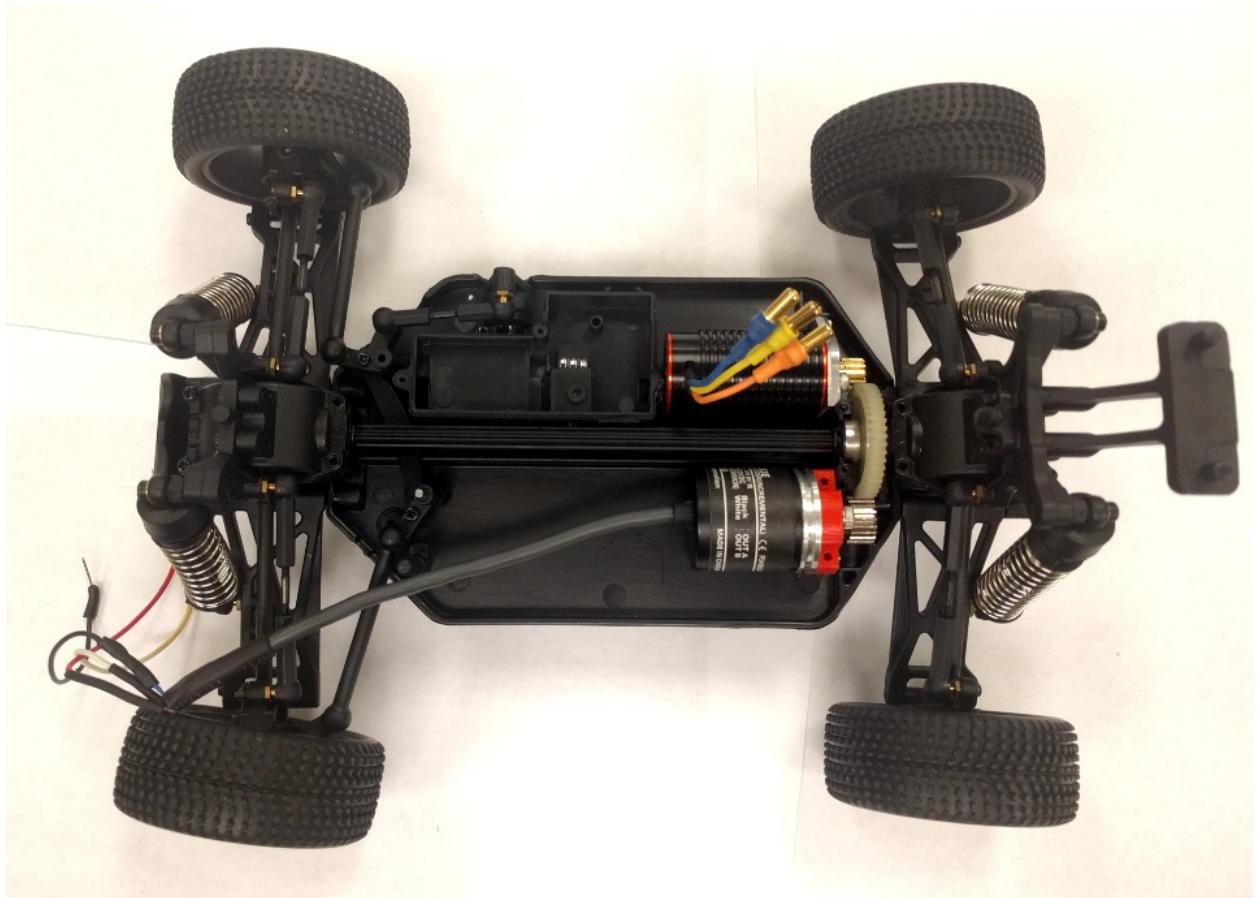
Fig. 8: Replaced the default motor with the TrackStar motor.
