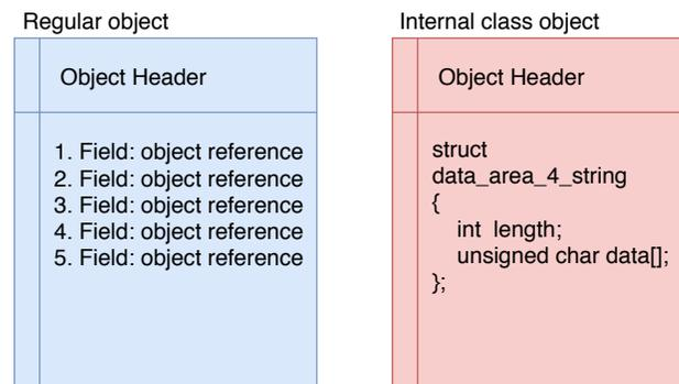
Fig. 2: Layout of regular and `.internal` class object
