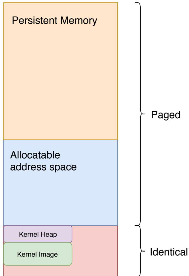
Fig. 1: Virtual memory layout for x86 architecture
