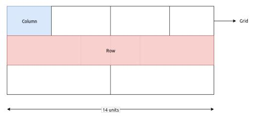
The grid system supports a maximum horizontal size of **14** units. For instance, 2 columns of width 7 units can be placed in a single row. Or a single column of width 14 units. If the width of the columns in a row exceed 14 units, the extra columns will automatically flow to the next row.
