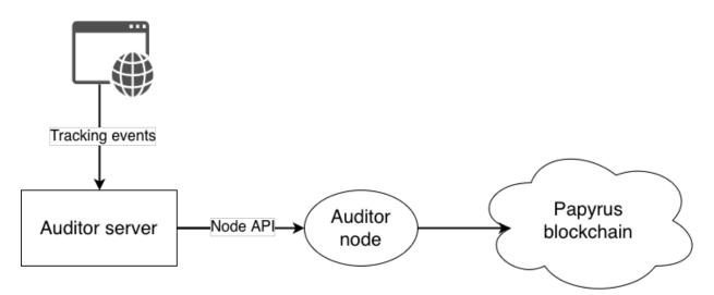
This case is the most diffucult for auditor, but it is the most effective solution. Auditor has to setup its own blockchain node and send logs to its API as in the previous case.
