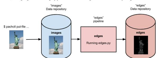
For now, we're going to create a single pipeline that takes in images and does some simple edge detection.
