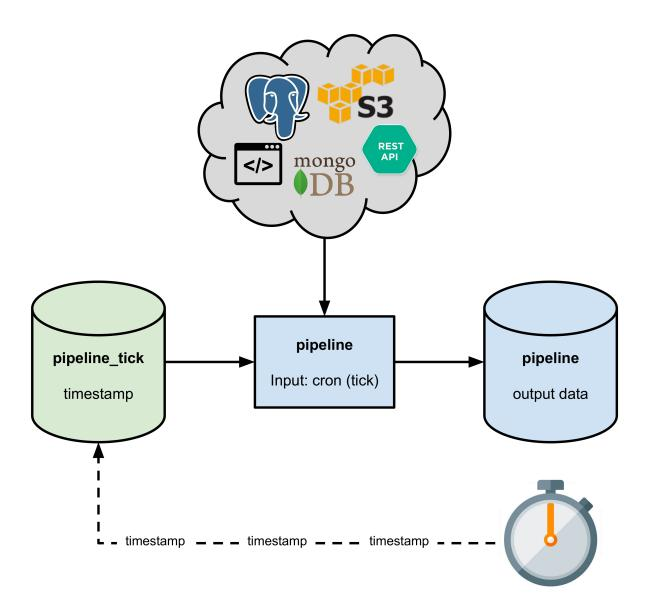
The pipeline will run every 10 seconds, querying our database and updating its output.
