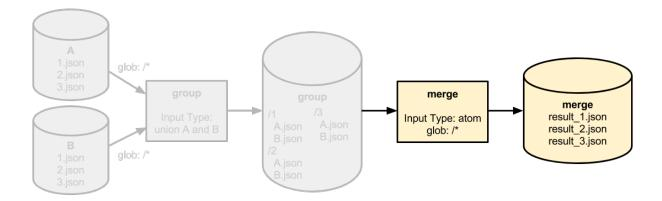
Once the records that need to be processed together are grouped by the first pipeline, our second pipeline can take the group repository as input with a glob pattern of /\*. This will let the second pipeline process each grouping of records in parallel.
