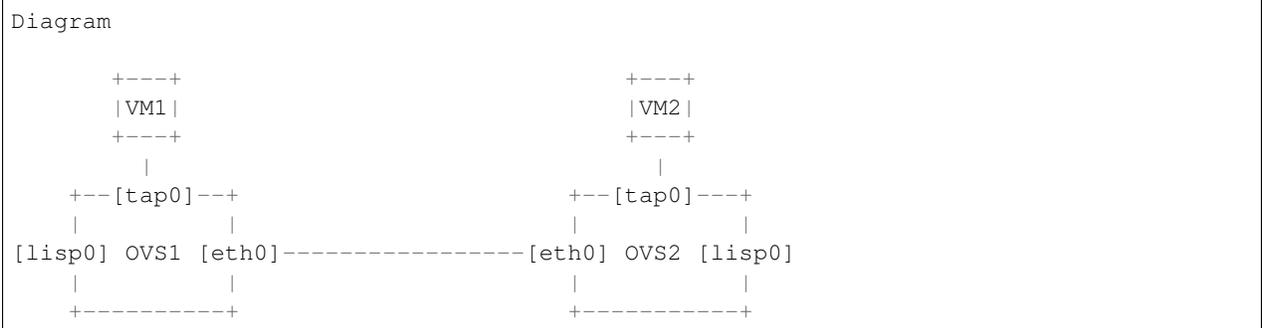
On each hypervisor, interfaces `tap0`, `eth0`, and `lisp0` are added to a single bridge instance, and become numbered 1, 2, and 3 respectively:
