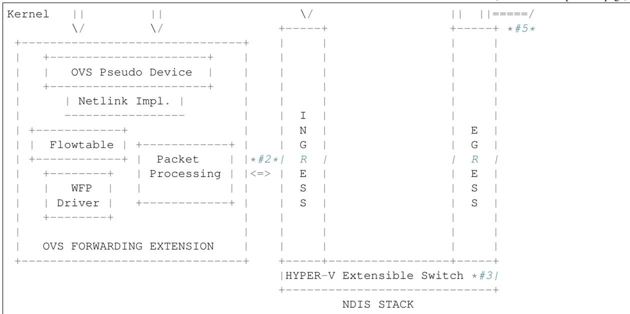
This diagram shows the various blocks involved in the OVS Windows implementation, along with some of the components available in the NDIS stack, and also the virtual machines. The workflow of a packet being transmitted from a VIF out and into another VIF and to a physical NIC is also shown. Later on in this section, we will discuss the flow of a packet at a high level.
