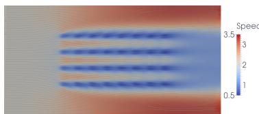
The power extraction by the farm (without taking losses into account) is 46 MW. This is 1.4 MW per turbine (32 turbines) which is unsatisfactory considering that placing a single turbine extracts 2.9 MW.
