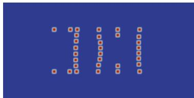
The optimization has arranged the turbines to “barrages” perpendicular to the flow. Furthermore, it added small north and east barrages of turbines that force the water to flow through the perpendicular “barrages”. The associated flow speed with streamlines is:
