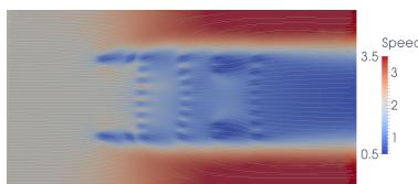
The power production of the optimised layout is 80 MW, or 2.5 MW per turbine. That is the optimisation increased the power production by 74 % compared to the initial layout!
