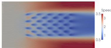
The power extraction by the farm (without taking losses into account) is 64 MW or 2.0 MW per turbine. Thats better but still non-optimal.
