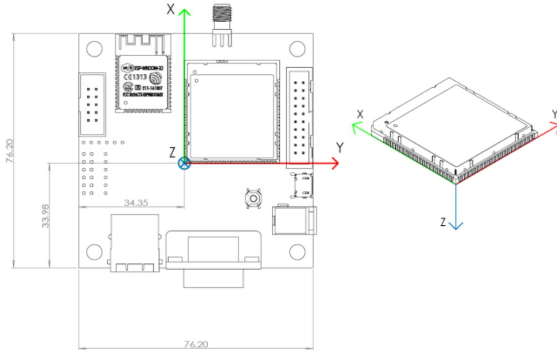
The following mechanical drawing shows the dimension (in mm) of the mounting plate for the OpenRTK330LI EVB:
