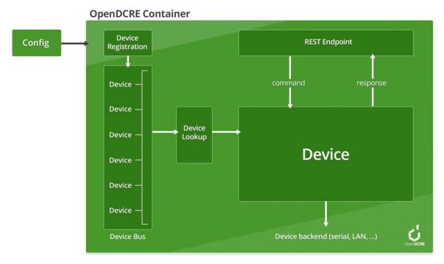
The OpenDCRE device bus is comprised of a set of boards and devices, individually addressable, and globally scannable for a real-time inventory of addressable devices. The OpenDCRE device bus allows devices to be read and written, and for various actions to be carried out, such as power control (on/off/cycle/status). Additionally, when a physical OpenDCRE device bus is not present, a software emulator can be used to simulate OpenDCRE API commands and functionality.
