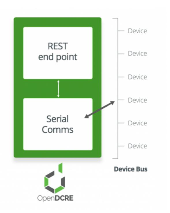
The OpenDCRE device bus is comprised of a set of boards and devices, individually addressable, and globally scannable for a real-time inventory of addressable devices attached to the bus. The OpenDCRE device bus allows devices to be read and written, and for various actions to be carried out, such as power control (on/off/cycle/status). Additionally, when a physical OpenDCRE device bus is not present, a software emulator can be used to simulate OpenDCRE API commands and functionality.
