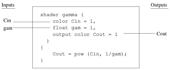
The shader's inputs and outputs are called *shader parameters*.
