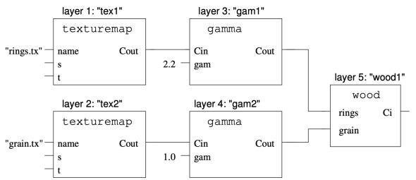
And here is sample pseudo-code shows how the above network may be assembled using an API in the renderer<sup>1</sup>:
